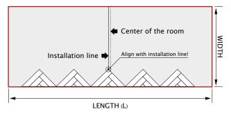
Lay out the triangles with their long side towards the starting wall. Align the centre triangle top with the installation line.
