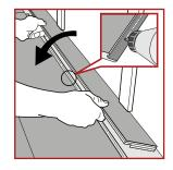
Remove the locking element according to the picture. Use a applicable glue to connect the strips. Pressplace wedges between the glued strip and the wall.
