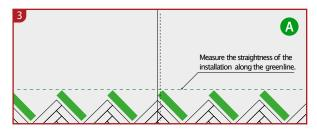
Install A-strips to connect all triangles. The joints between the A-strip and the triangle need to be checked very carefully. No protruding edge may be felt!
