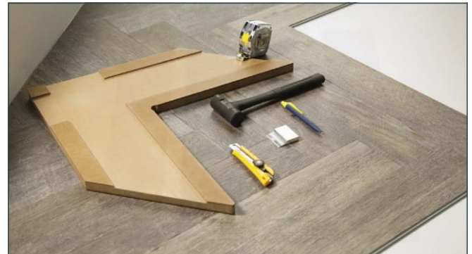
Preparation Tools needed: a tape measure, pen, cutter knife, T-square, soft rubber mallet, disassembling wedge.
