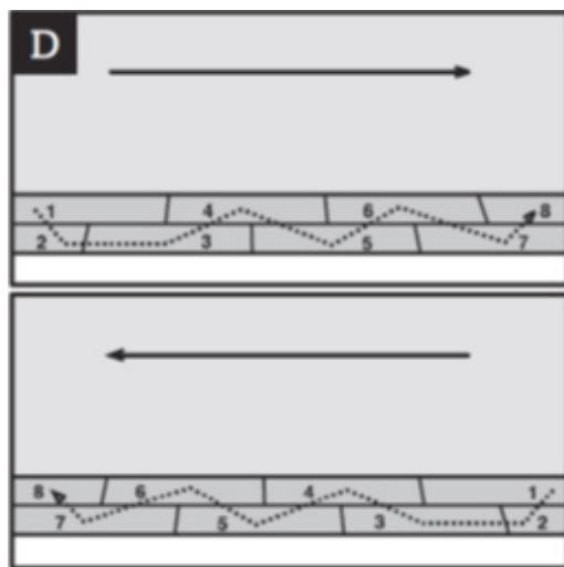
4. When starting your first two rows, lock planks #1 & #2 (Note plank #2 has been cut shorter in length) in place by angling the plank's tongue and groove at an angle just enough to get your fingers underneath the plank. Angling the planks any higher makes it hard to get a good tight seam. You will know when the planks are fully locked when the planks lay flat on the subfloor. Using a tapping block on the
