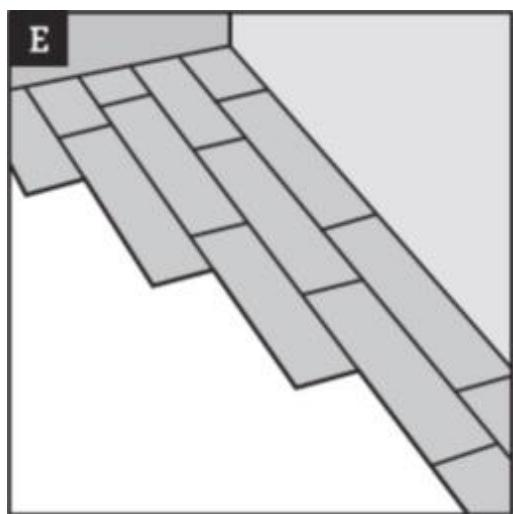
7. Fitting around irregular objects is no problem. Simply make a pattern out of heavy paper to fit around pipes or irregular objects. Place the pattern upon the plank and trace. Cut along trace lines using a
