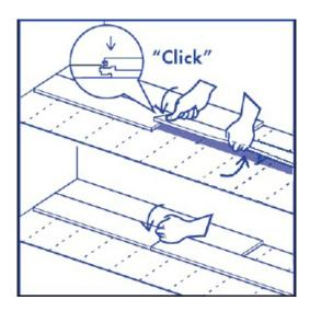
8. Now connect the panels of the first two rows on the short sides. Check the expansion gap of and make sure the first rows are on a perfect straight line. You can check this by holding a thin rope along the installed planks and adjust the straightness of your floor when necessary. An expansion gap of 8 mm along the perimeter should be maintained. In the width and in the length direction of the planks there is no need for extra expansion gaps.
