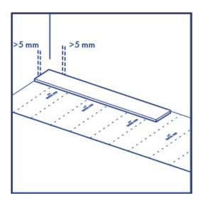
5. Supremo Rigid Core can easily be cut using a cutter or utility knife with the decor side face up. When cutting the vinyl plank, mark the line and use the knife to make a firm cut
