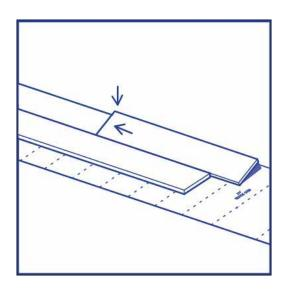
9. Continue the installation like this row by row towards the end of the room. Always check each joint before continuing. You can press down gently with your thumb on top
