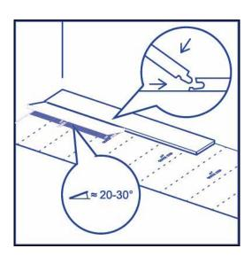
7. Then slide the third plank together horizontally. Slightly lift the plank to be installed by holding your hand underneath. Push the short side joint down gently with your thumb moving from the inner corner towards the outside until you hear a "click". Ensure the short side ends are closed by knocking gently on the short side click connection with your wrist. Don't use a hammer or tapping block as it may possible harm your click con-
