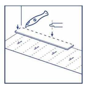
4. Fit the plank with cut off sides against the walls. Make sure that you leave an expansion joint of 5 mm. For installations with floor heating, we recommend to leave an expansion gap of 10 mm.
