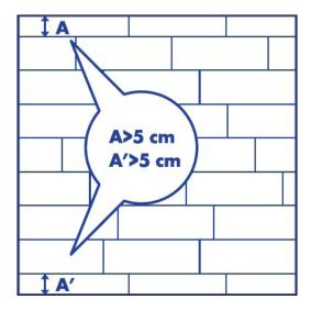
2. During installation, make sure that you mix up the floor panels sufficiently so that there are not too many identical, lighter or darker panels next to each other. To obtain the best visual effect, it is best to fit the panels in the direction of the longest wall and parallel to the incidence of light. Ensure that the end joints of the panels in 2 successive rows are never in line, they should be staggered by at least 30 cm.
