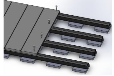
Attention: The WPC products' expansion rate is around 0.3% to 0.5% depends on deck length and weather condition in different places. Based on this expansion rate, there must be a gap (at least 1mm) always between two decks.
