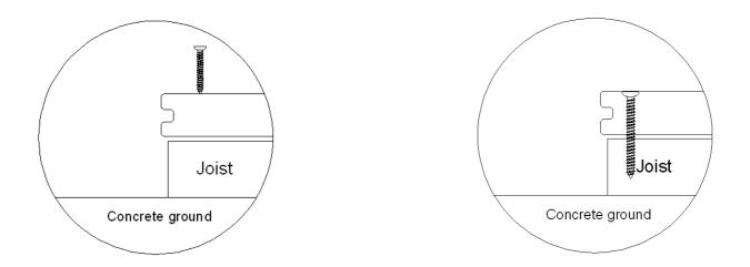
After the first deck is fixed, the rest decks to be fixed by screws and clips in turn
