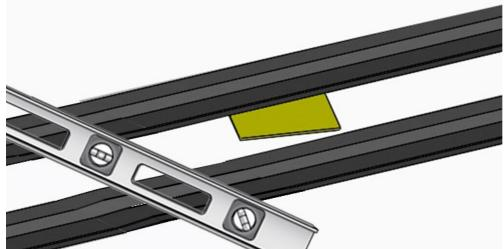
Attention: it is required that the deck surface is mounted flat and no water can collect on the surface or in the chambers. If water collects in the chambers for a long period, the board may start cupping and waving because of the moisture expansion.
