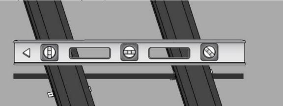
If the joists level is not smooth, please ajust the level by filling the gap between the joist and ground with slices.
